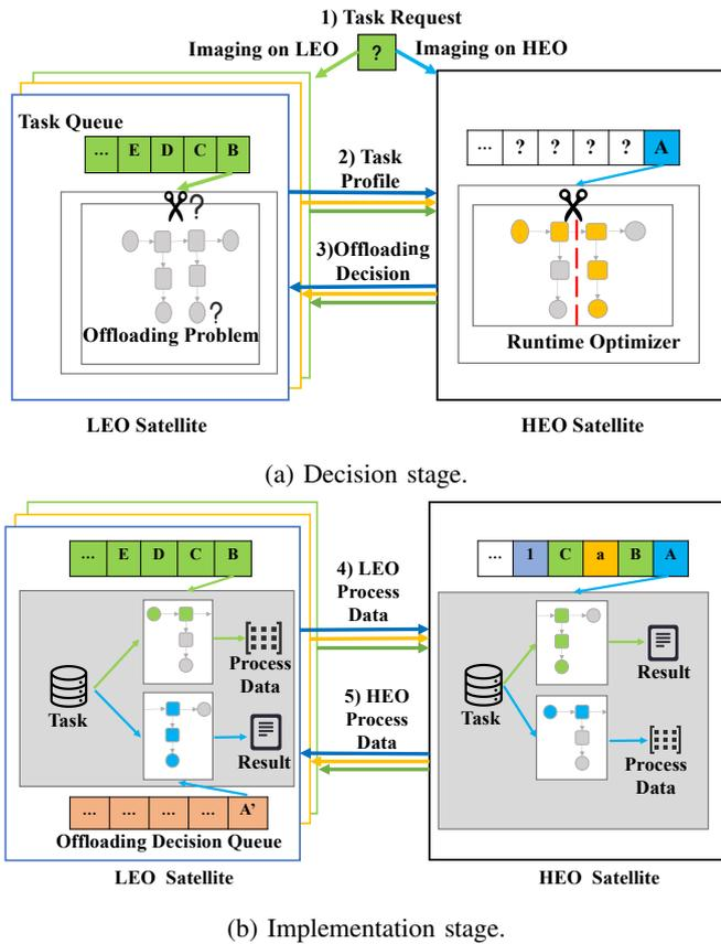
Fig. 1: The workflow of collaborative task stream offloading system.
